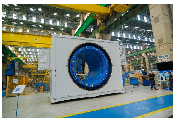
Manufacturing of synchronous condensers at the ANDRITZ facility in Araraquara, Brazil
